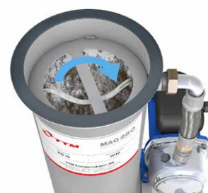
3. Press down and rotate the locking ring until the grooves match the lugs.
